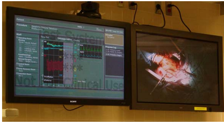
Fig. 4 The integrated OR data display resides directly adjacent to the surgical display. The close proximity of two large displays mandated that the design avoid detracting from the pre-existing surgical display, which is often in use during cases. The surgical display provides the entire OR team with an overview of the surgical situation. The OR data integration system is designed to provide a similar overview for key
